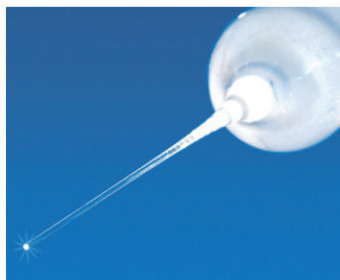
Large RIC preform for the production of optical fibers. Image by Heraeus Holding GmbH
