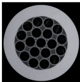
End-view image of a fused 19:1 fiber combiners. Image by Vytran LLC
